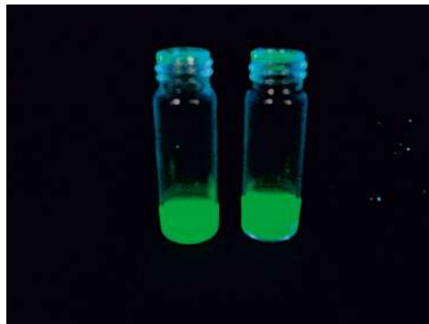
Fig. IV.13-5: Quantum dots, of Manganese doped under 254 nm UV light
