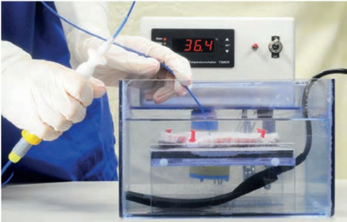
Fig. 1: In-vitro RF ablation experiments on pork in the wetlab containing physiological saline solution, heated to body temperature and simulating the cooling influence of the blood flow
